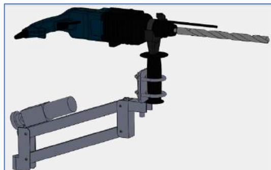
Figure 1: Proof of concept clamping design.
