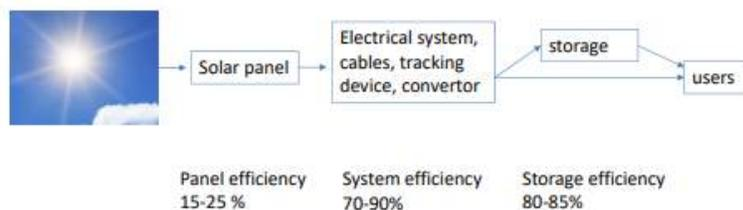
Figure 4 Energy process supply to the shelter
