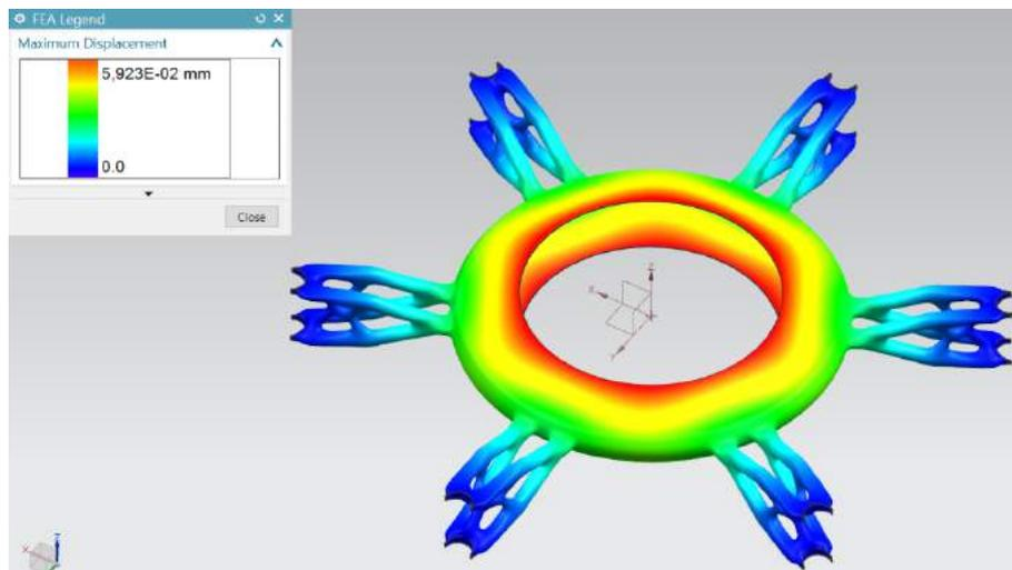
Figure 4 the maximum and minimum displacement of the drone body in [mm]
