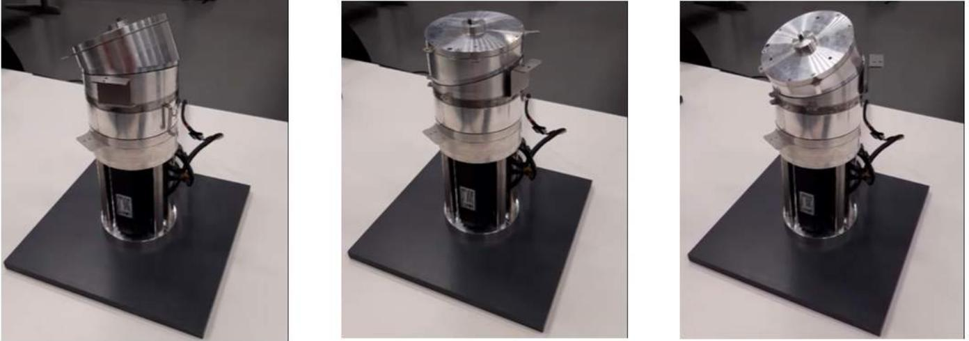
**Fig. 1:** The different tilt angles of the (previous) SmartWrist
