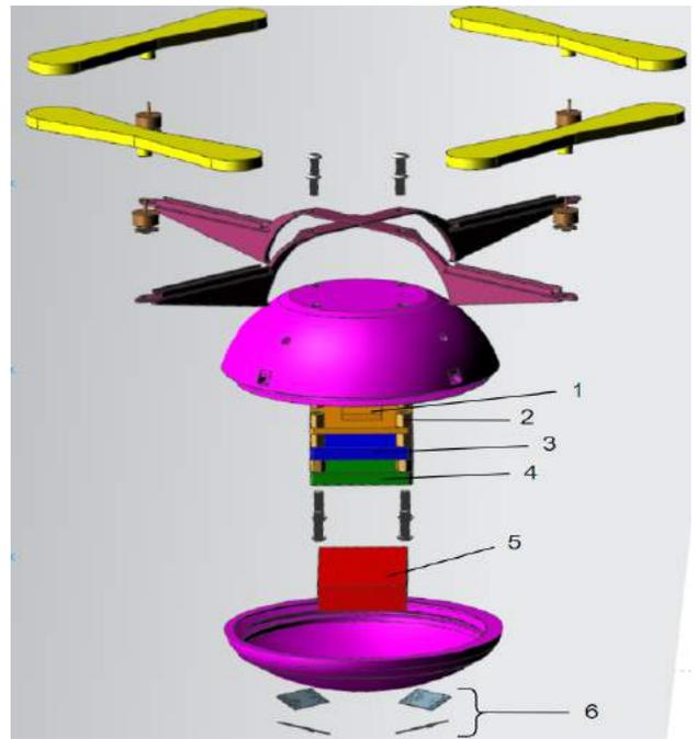
Figure 9 (Exploded view of quadcopter)
