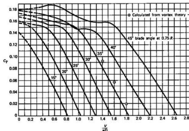
Figure 2 Typical propeller thrust curves as a function of advance ratio ( $J=v/nD$ ) and blade angle [4]
