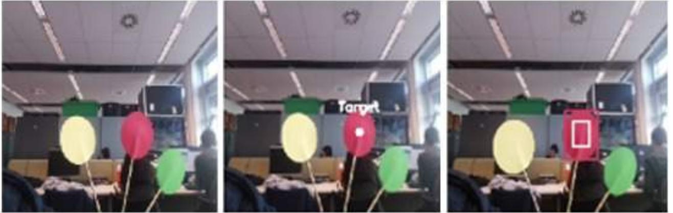
**Fig. 5:** Original Image (Left), Detection Result (Middle), Tracking Result (Right)
