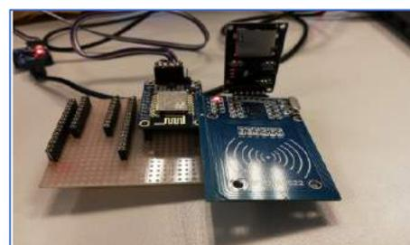
Figure 4: ESP8266, SD card, RFID comprising a circuit for the wireless communication between the server and interface.
