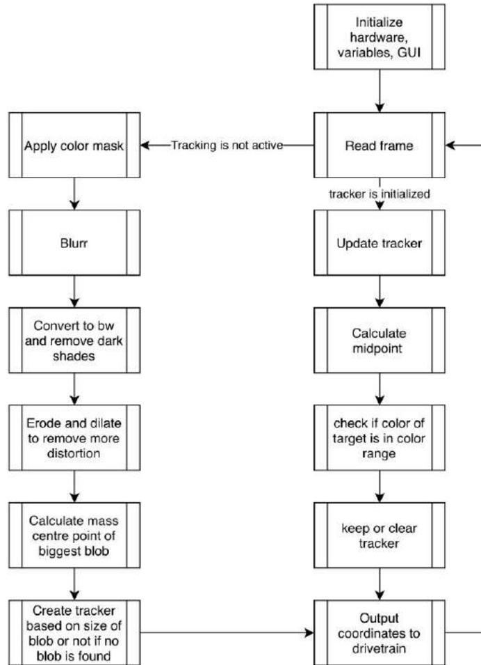
Fig. 3: Compact Flowchart of the Vision Software
