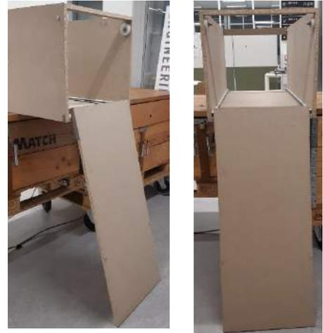
Once the e-step is attached, the sliding board moves from the vertical position, to horizontal (which must be done by the user).
