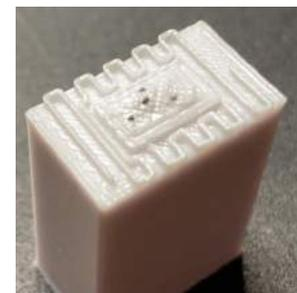
Figure 7: Tested subject with four wires. Part failed above the wire location.
