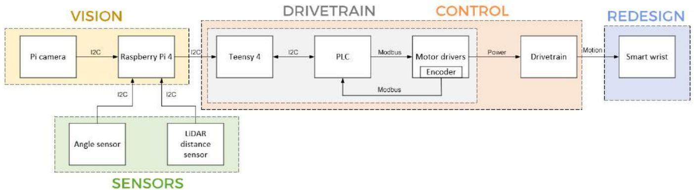
**Fig. 2:** Total Architecture and Communication
