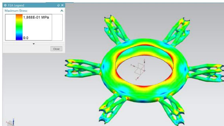
Figure 5 the maximum and minimum stress within the drone in [MPa]
