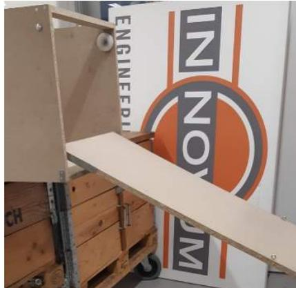
After this, the board is slid into the main storage unit, where it will be protected from weather and theft. The sliding board has a stopper at the back, which stops it from going too far.
