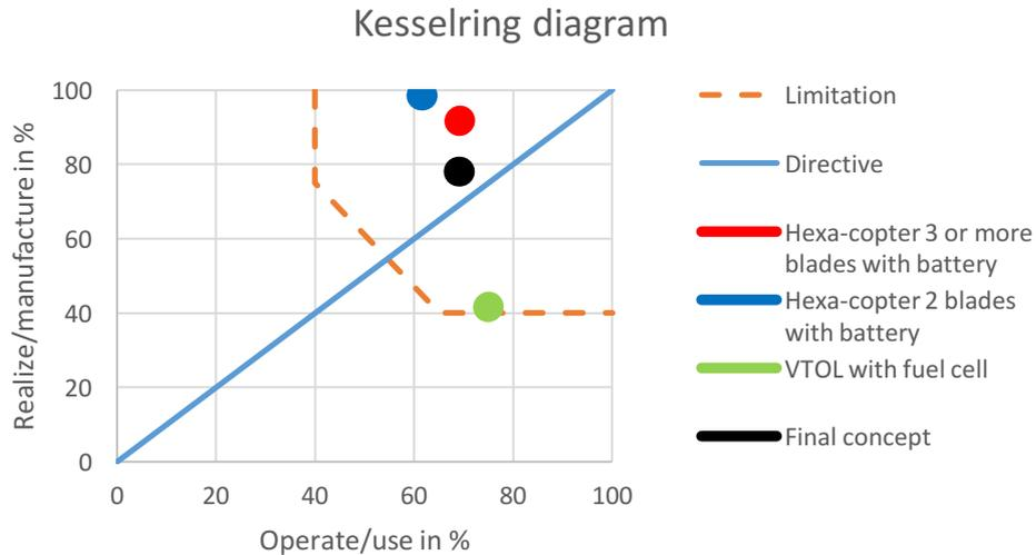
Figure 1 Kesselring diagram for 3 concepts
