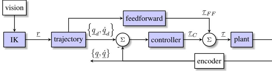
**Fig. 5:** Overview of the control architecture of the SmartWrist. Purple colored boxes are covered in this paper.
