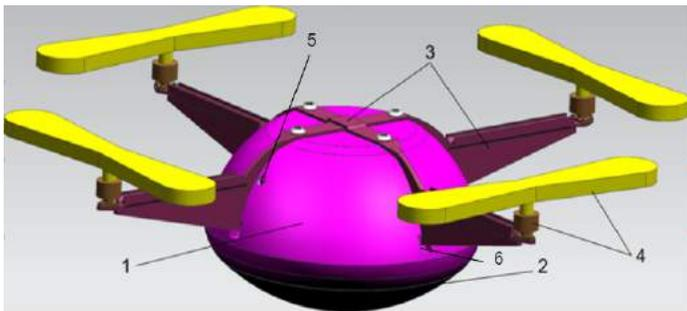
Figure 7 (Quadcopter. 1 Main frame; 2 Bottom Part; 3 Arms; 4 Motors and Propellers; 5 Wire holes; 6 Claw grip)
