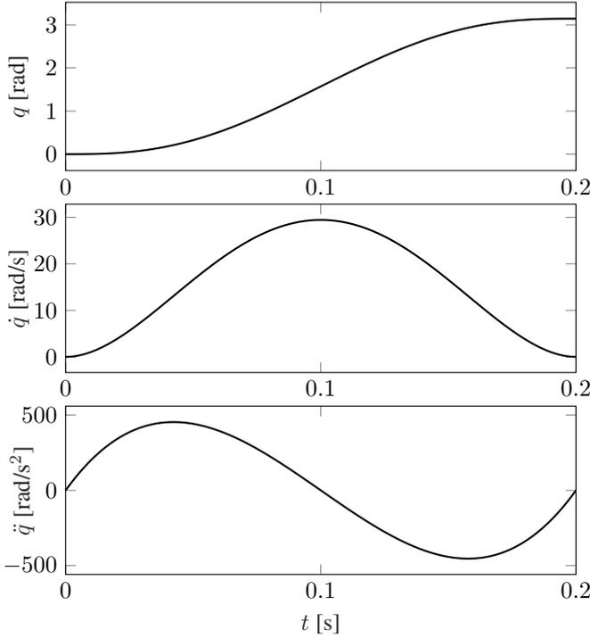
**Fig. 6:** The quantic polynomials solve the discontinuity of the acceleration. Herein, the jerk is still a second-order polynomial.
