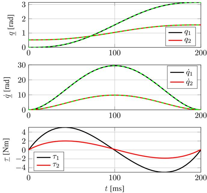
**Fig. 7:** The simulation results for the controller as described in (11). Green dashed line represents the quantic polynomial tracking.
