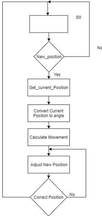
Fig. 4: Flowchart of Drivetrain Software
