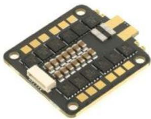
Figure 6 (32Bit ESC)
