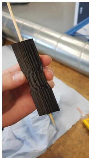
Figure 12: Test sample with a glued bamboo skewer in the printed base sample
