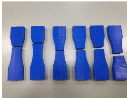
Figure 1: Test samples with reinforcing metal needles injected into the vertical centre axle.
