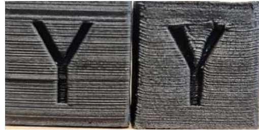
Figure 7 One side of the printed test cubes. on the left the finalized cubes, on the right the first attempt
