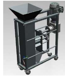
Figure 3, Dispensing Unit, the subsystem that divides the ingredients into portions.
