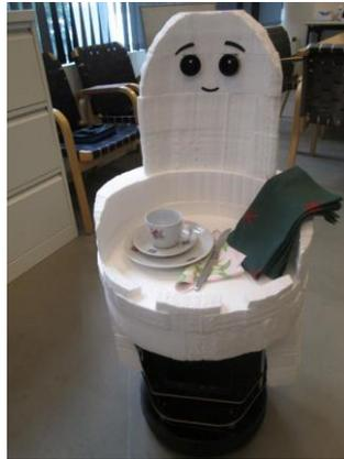
**Fig. 1.** This is Casper. It is a low-fidelity prototype, coated in styrofoam and equipped with a pair of eyes made from bottle caps. The robot is a Turtlebot 2 on a Yujin Kobuki mobile base.
